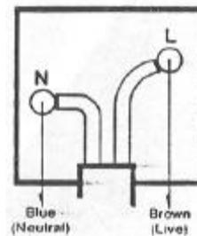
Do not connect any wire to the larger pin marked E or down when wiring a plug. Ensure that all terminals are securely tightened and that no loose strands of wire exist.
